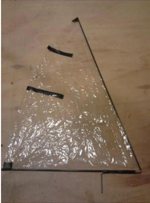
I copied the sail dimensions from the Footy forum and drew a sail shape onto card. 3mm carbon tube was used for the mast and boom, whilst I made the sail from a freezer bag. The front of the sail was made 20mm too long, allowing it to be turned back on itself and secured with clear double sided tape. Thus forming a loop into which the mast could be inserted. The head and the foot of the sail were secured using insulating tape.
